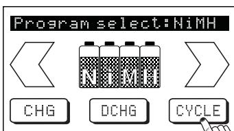
**Note:** if the voltage of the battery is lower than 2.5 V (single-cell), the Delta-Peak voltage may not be detected properly, which may result in an overcharge.
