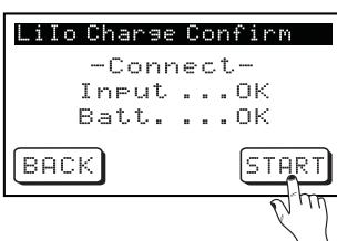
After connecting the battery and press **START** once, the charger is checking the battery and displays **OK**.
