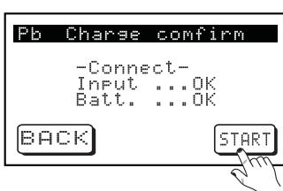
After connecting the battery and press **START** once, the charger is checking the battery and displays OK. To start the charging process press **START**, to stop and check the settings again press **BACK**.
