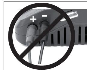
**⚠ WARNING:** Use only batteries with XH balancer plugs. Never try to connect other plug types with the charger! **The plug or charger may damage or worse, the battery catches fire or explodes!** If necessary, use a suitable adapter cable.
